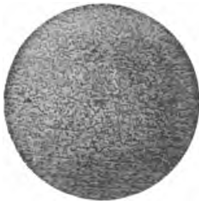
PHOTOMICROGRAPH, CARBON STEEL INGOT. LONGITUDINAL SECTION 2 1/2 IN. FROM BOTTOM OF INGOT, 1 1/4 IN. FROM EDGE. MAGNIFICATION 5 DIAMETERS.
